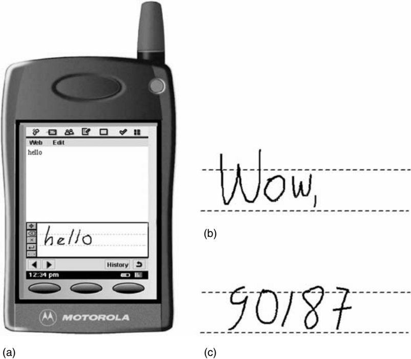
FIGURE 26.38 Word-based text input method for mobile devices. In (a), a user interface prototype. In (b), an image of the mixed-case word Wow, where relative size information can be used for distinguishing among the letters in the Ww pair. In (c), an image of the digit string 90187 where ambiguity in the identity of the first three letters can be resolved after identifying the last two characters as digits.
