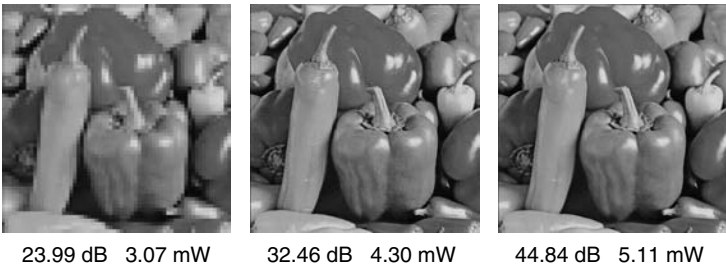
FIGURE 13.12 Compressed image quality and power. (From Xanthopoulos, T. and Chandrakasan, A., IEEE Journal of Solid-State Circuits , 35(5), 740, May 2000. With permission.)
